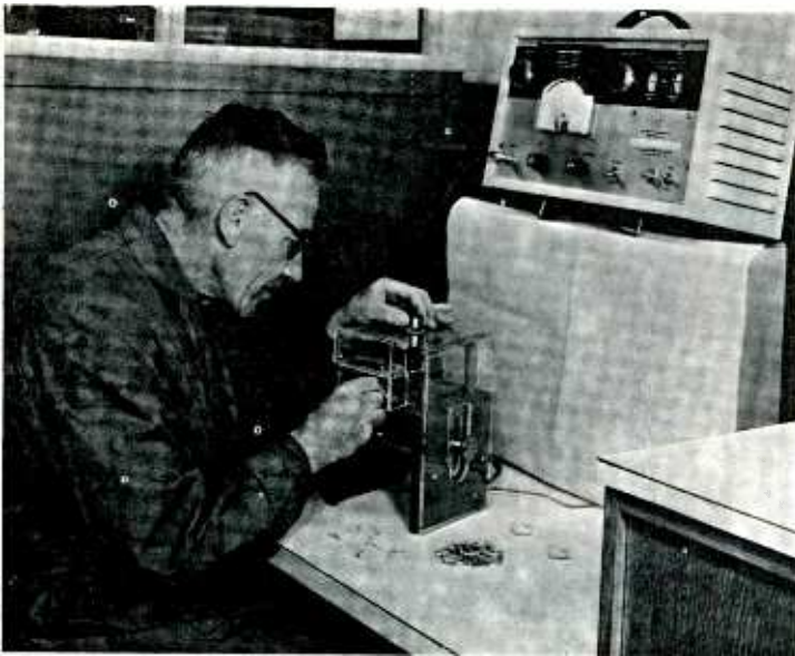
Beta-ray backscatter apparatus being used by ultra Electronics (Components) Limited to measure the thickness of precious metal plating in production processes
